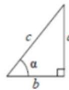
$$\begin{aligned}\sin \alpha &= \frac{a}{c} \\ \cos \alpha &= \frac{b}{c} \\ \operatorname{tg} \alpha &= \frac{a}{b}\end{aligned}$$
