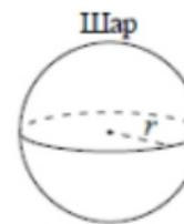
$$\begin{aligned} V &= \frac{4}{3}\pi r^3 \\ S &= 4\pi r^2 \end{aligned}$$
