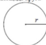
$$\begin{aligned} C &= 2\pi r \\ S &= \pi r^2 \end{aligned}$$
