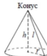
$$\begin{aligned} V &= \frac{1}{3}\pi r^2 h \\ S_{\text{бок}} &= \pi r l \end{aligned}$$
