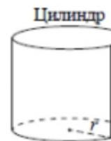
$$\begin{aligned} V &= \pi r^2 h \\ S_{\text{бок}} &= 2\pi r h \end{aligned}$$
